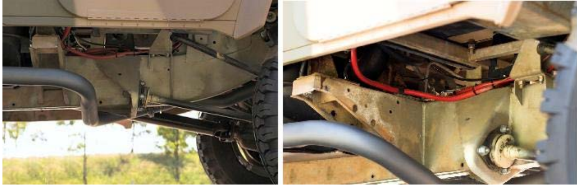
Figure 112A-16: SFPV's Electrical Wiring
