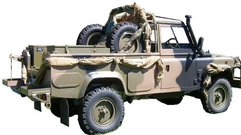
Figure 112A–4: Surveillance Variant - Canopy and Rear Seat Removed
