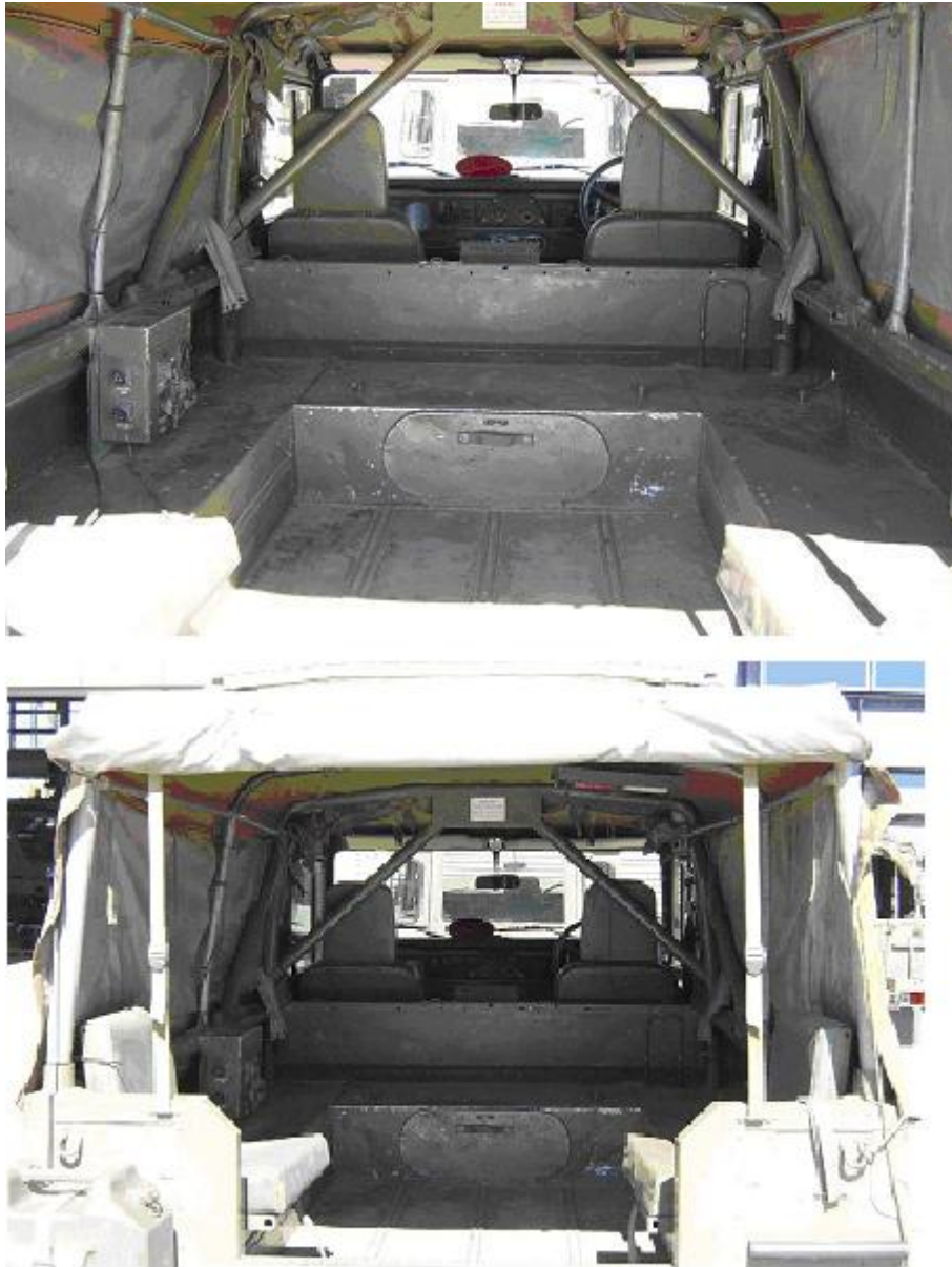
Figure 112C-5: FFR Variant Interior – Radios Unfitted
