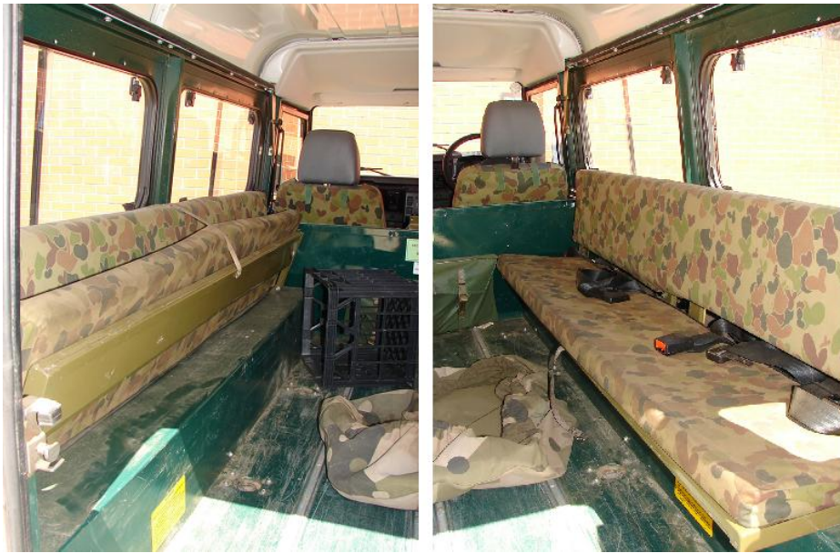
Figure 112G-11: Land Rover 4x4 Defender 110 TD5 Rear Interior Seating Stowed (Left) and Down (Right) Positions
