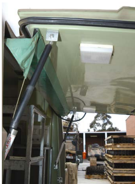
Figure 113D-7: General Maintenance Vehicle Side Access Dust and Weather Seals, and Work Lights
