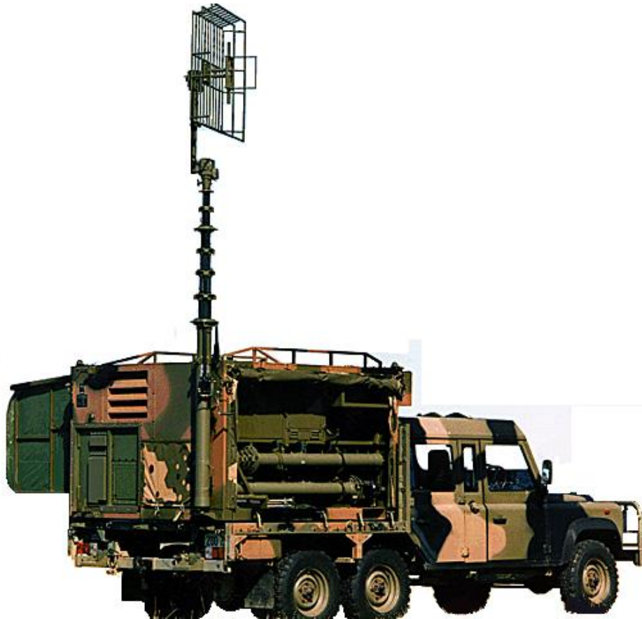
Figure 113F–1: Radio Relay Assemblage with Antenna Erected
