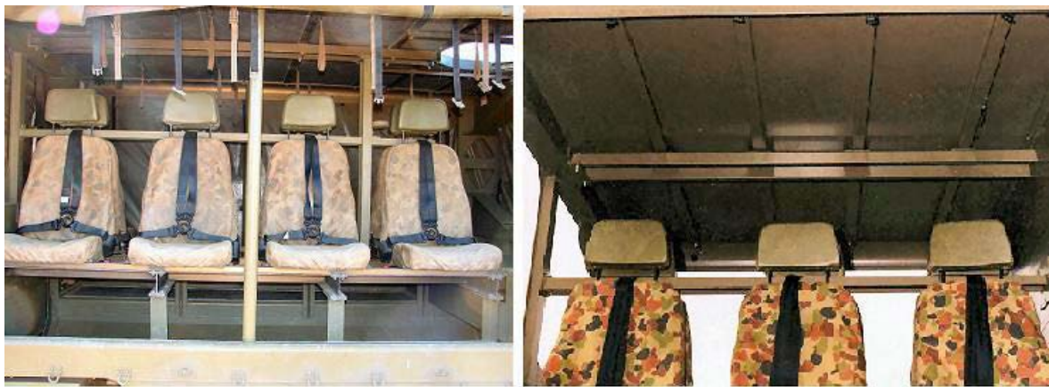
1130-5: Infantry Mobility Variant Rear Seating Floor Area (Left) and Roof Area (Right)
