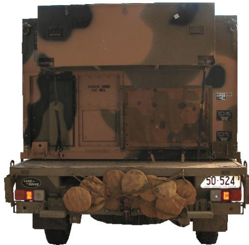
Figure 113F-3: Radio Relay Assemblage Rear
