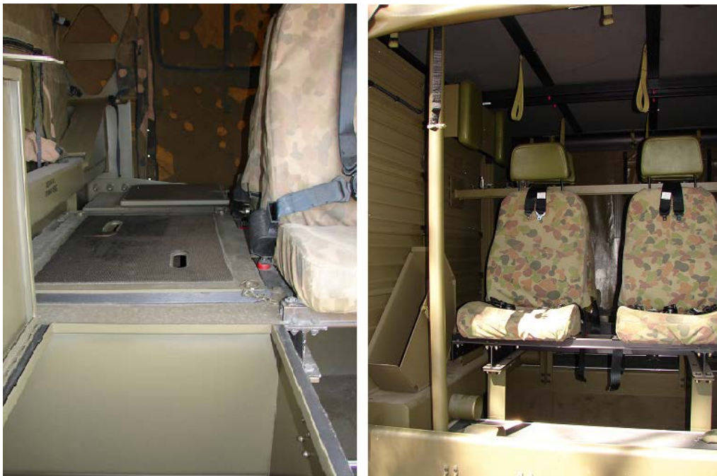
Figure 113J-4: Assault Pioneer Vehicle Rear Storage Compartments (Left) and Rear Compartment Wall Fittings (Right)
