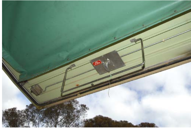
Figure 113D–8: General Maintenance Vehicle Dust, Weather Seals, and Blackout Curtain
