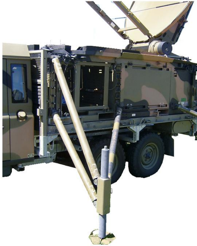
Figure 113E–4: Landrover 6X6 SATCOM Terminal Assemblage (Parakeet) Supports and Stands
