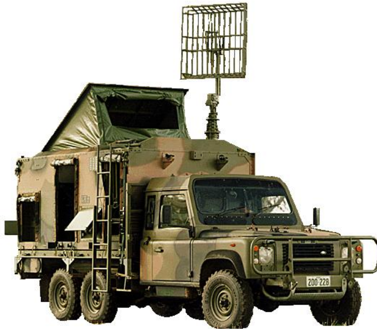
Figure 113K-1: Circuit Switch Assemblage
