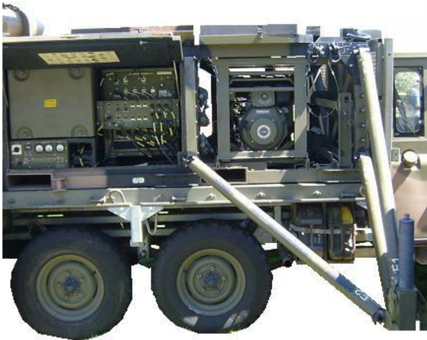
Figure 113E-3: Landrover 6X6 SATCOM Terminal Assemblage (Parakeet) Electronic Compartments
