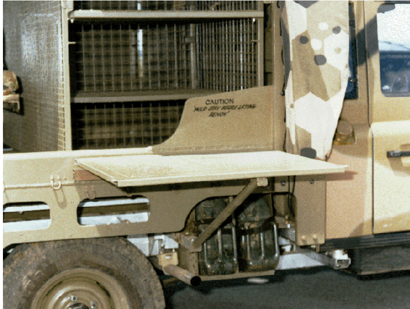
Figure 113P-7: Direct Fire Weapons Vehicle Forward Storage Cages, Door Opened
