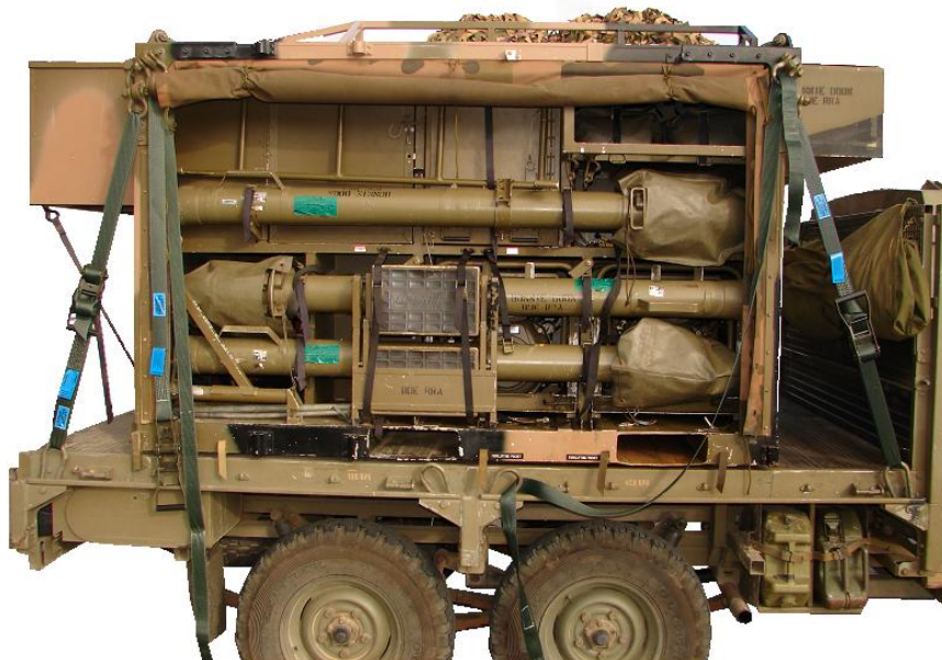
Figure 113F-5: Radio Relay Assemblage Antennae Storage Area
