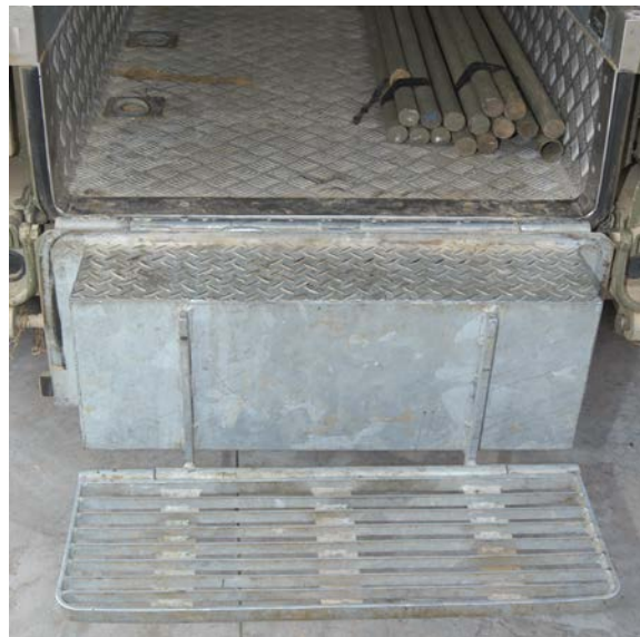
Figure 113C-8: Typical Module Step Well Seal
