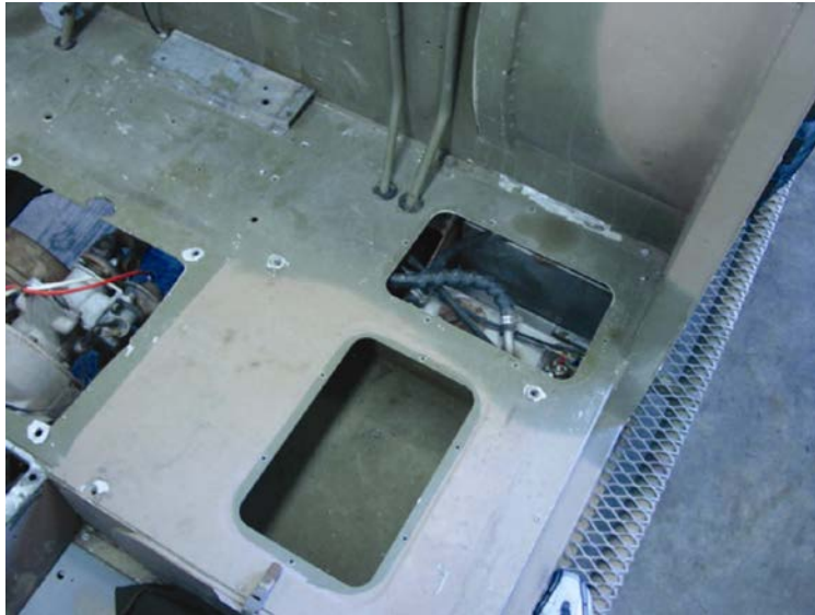
Figure 113G-6: Landrover 110 6x6 Long Range Patrol Vehicle Passengers Side Under-seat Storage Bin
