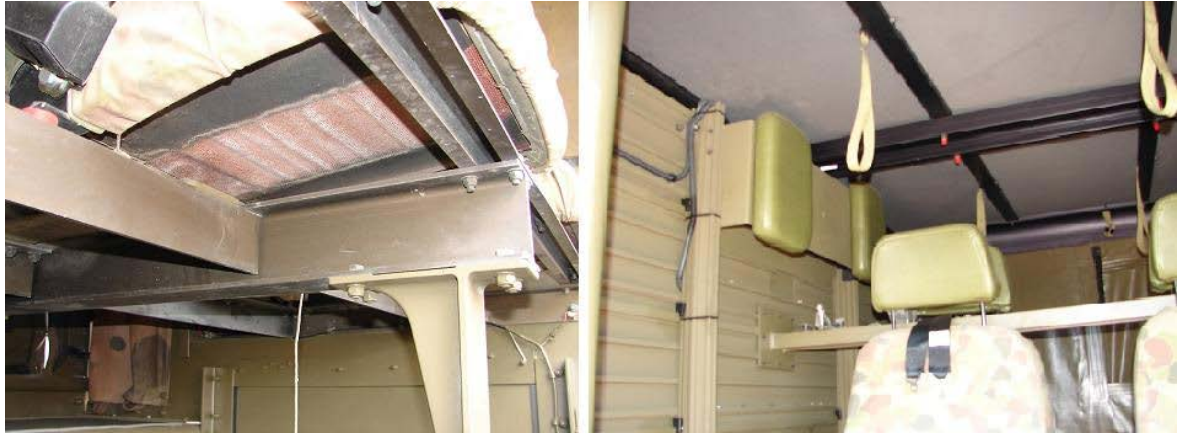
Figure 113J-5: Assault Pioneer Vehicle Under Rear Seats (Left) and Head Side Pads (Right)
