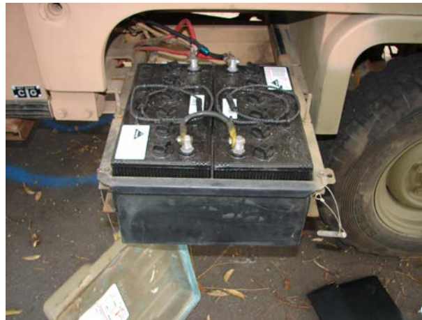
Figure 113A-5: Ambulance Battery Bay
