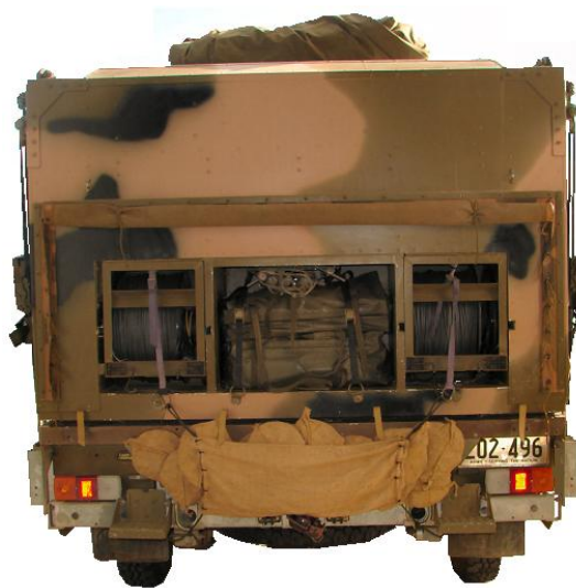
Figure 113K-4: Circuit Switch Assemblage Rear Stowage Compartments
