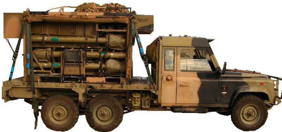
Figure 113F-4: Radio Relay Assemblage Side Covers Open
