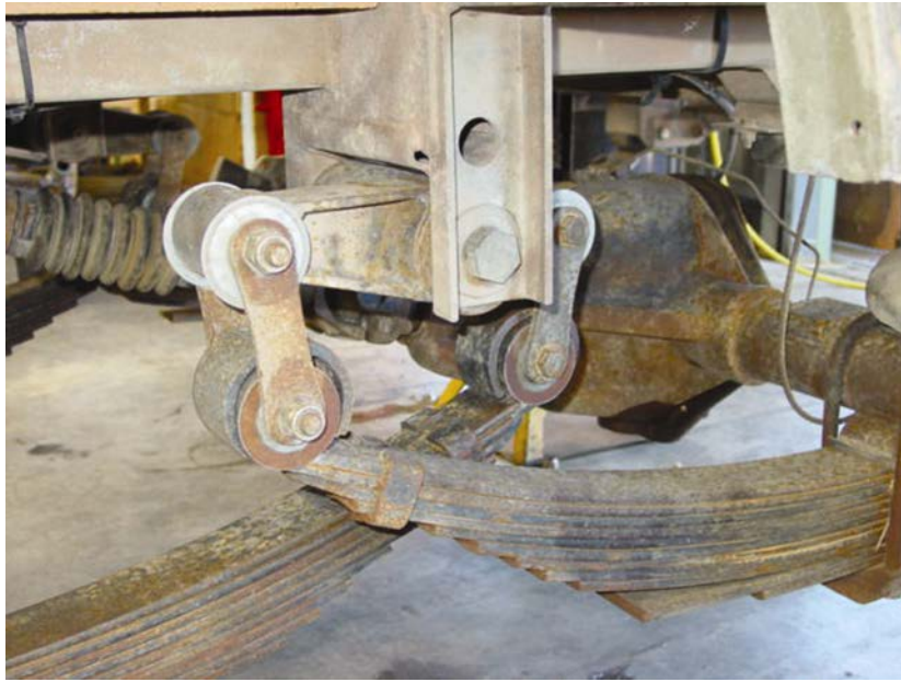
Figure 113G-14: Landrover 110 6x6 Long Range Patrol Vehicle Rear Suspension Rocker Beam Mount to Chassis
