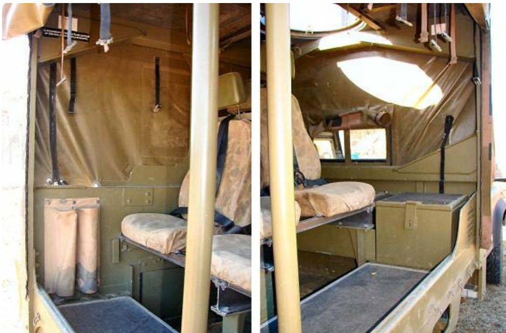
1130-7: Infantry Mobility Variant Wall Holders (Left) and Stowage Bin (Right)
