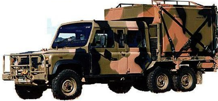
Figure 113F-2: Radio Relay Assemblage
