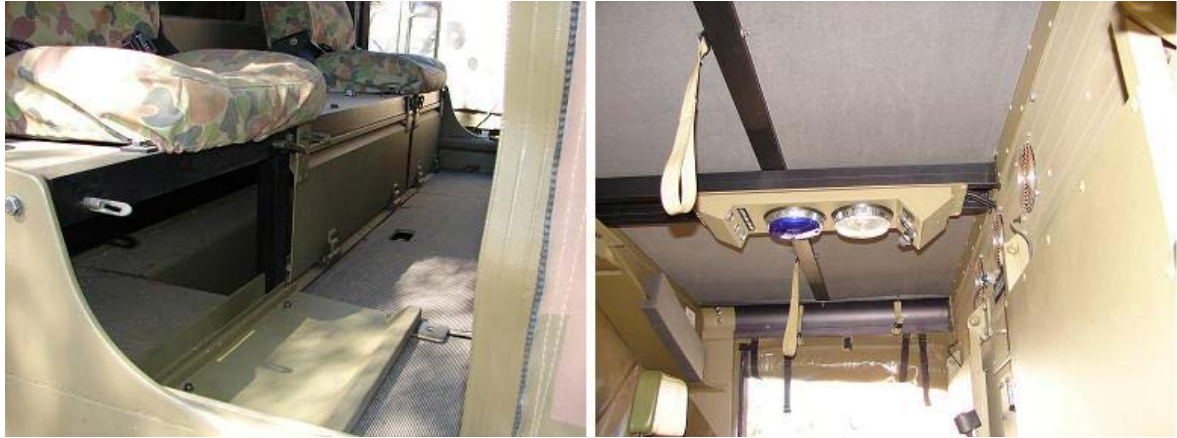
Figure 113J-8: Assault Pioneer Vehicle Forward Compartment Under Seat Stowage (Left) and Light Fittings (Right)
