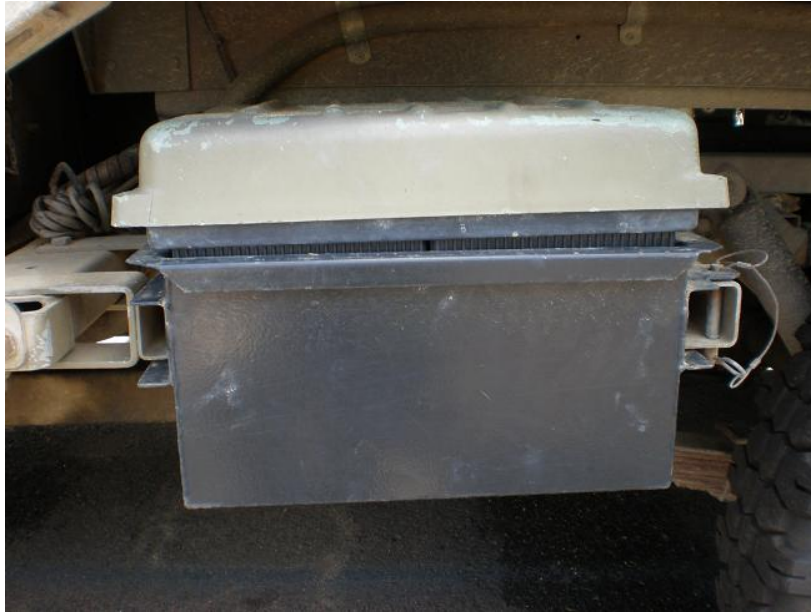
Figure 113Q-2: Land Rover 6X6 Fitted for Radio Battery Bay
