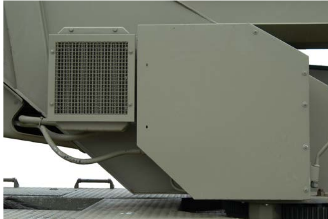
Figure 32A-6: Tadano's Hydraulic Oil Cooler
