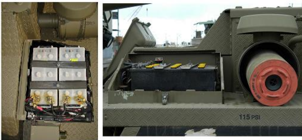
Figure 32A-33: Tadano's Battery Box & Air Cleaner
