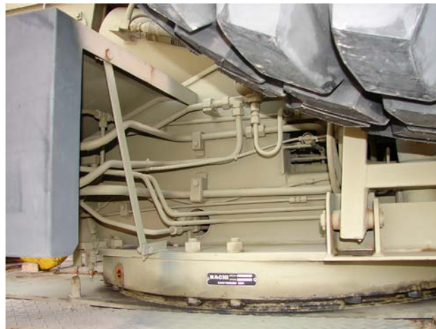
Figure 32B-6: Tadano's Crane Turntable
