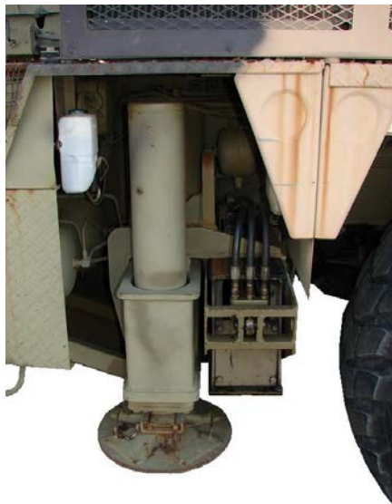
Figure 32B-11: Tadano's Outrigger Stabiliser Stand
