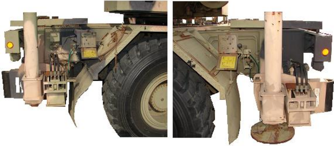
Figure 32B-12: Rear Stabilisers - Foot Removed (Left), Foot Fitted (Right)
