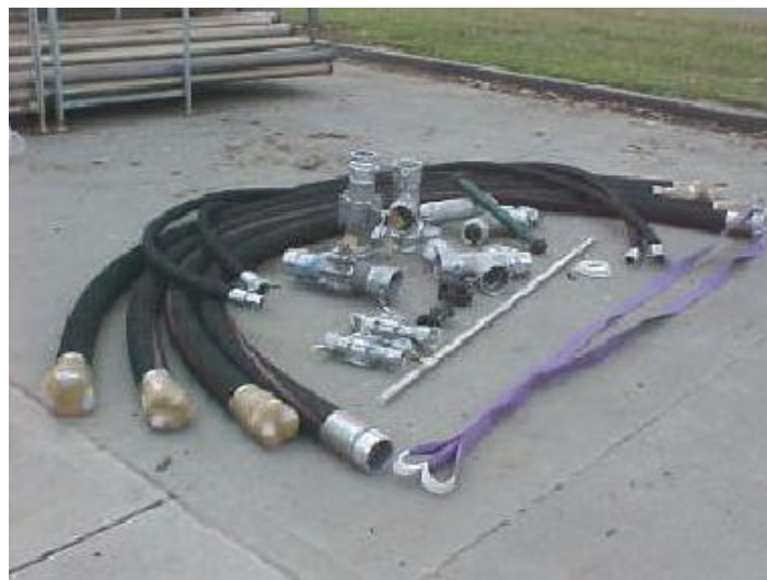
Figure 33B-3: Tank, Fabric, Collapsible Fuel Piping and Components
