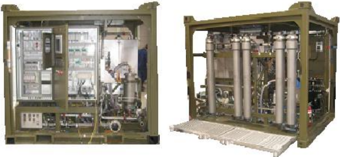
Figure 34C–1: Water Purification Unit ISO 1D container - 400,000 litres External Areas
