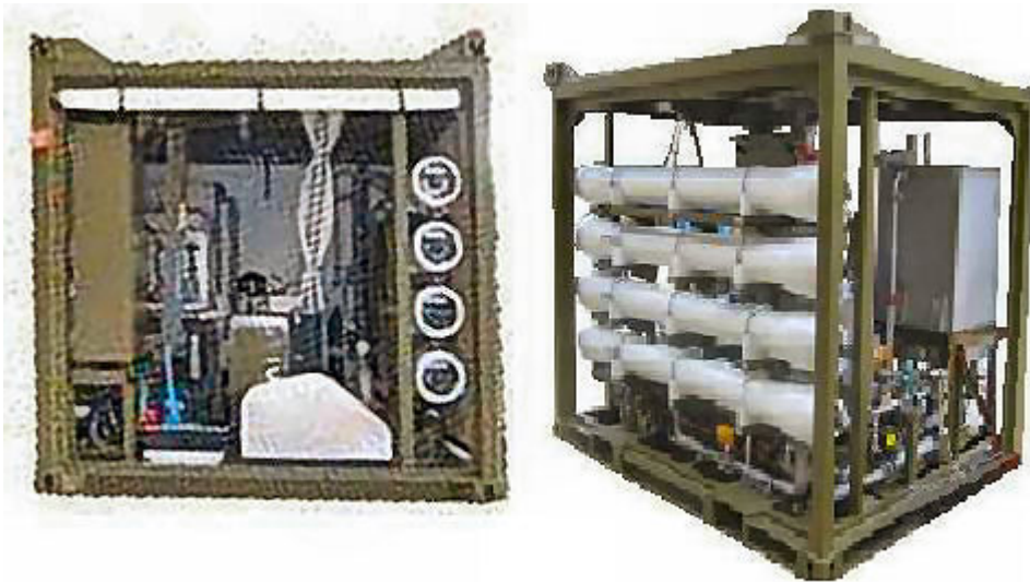
Figure 34D-1: Water Purification Unit Reverse Osmosis (Medium) ISO 1D Container - 100,000 litres External Areas
