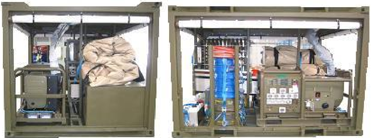
Figure 34E-1: Water Purification Unit Equipment Storage Units ISO 1D container's External Areas
