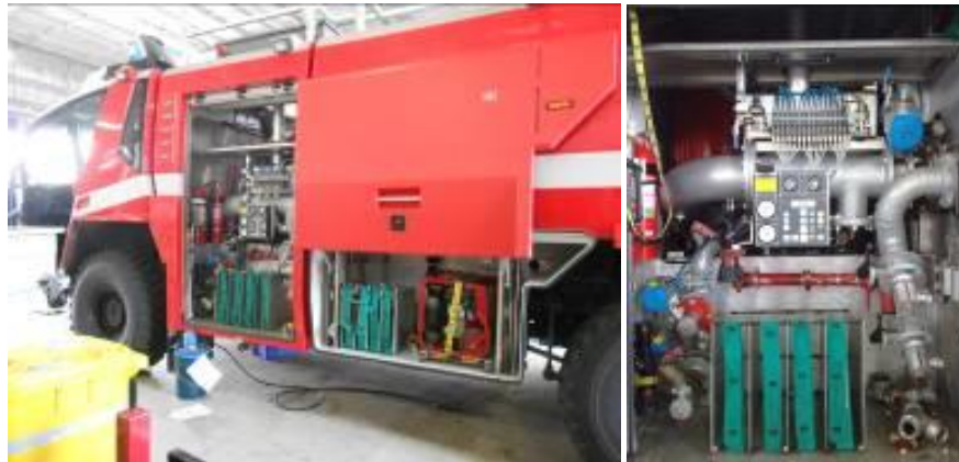
Figure 47A-14: Forward and middle passenger side locker compartments and forward passenger side locker
