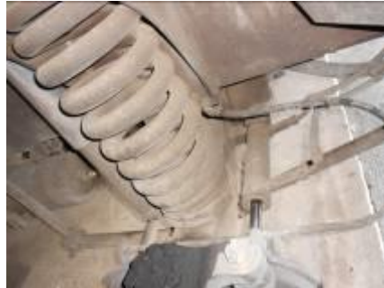
Figure 47A-11: Panther's suspension spring
