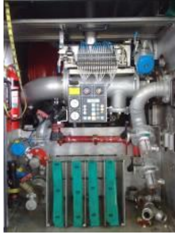
Figure 47A-2: Panther's Hoses Connection and Pump Panel
