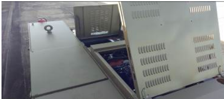
Figure 48D-11: TUG U30 Top Panels – Battery (Rear) and Engine (Front)
