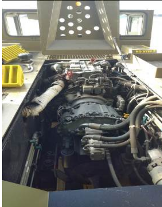
Figure 48C-8: SCHOPF F110 Tow Motor – Engine Compartment Top Panels Open
