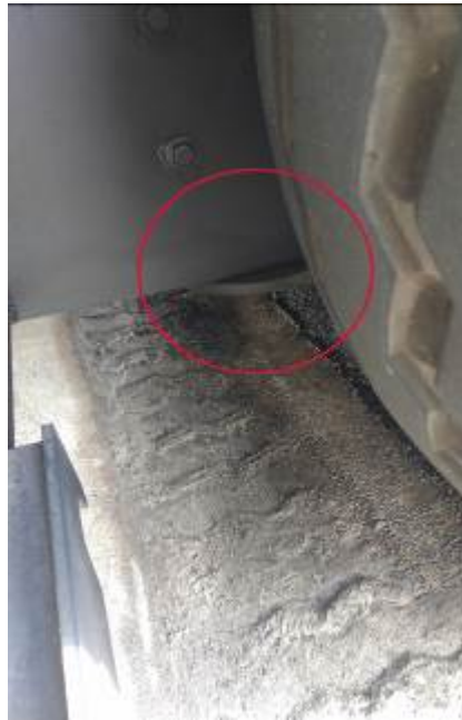
Figure 48D-6: TUG U30 Tow Motor - Internal Jacking Pads (Circled)
