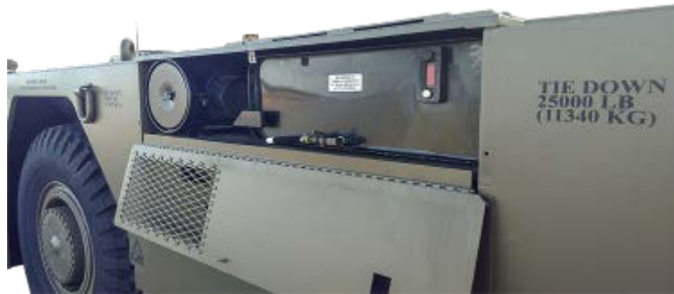
Figure 48D-7: TUG U30 Left Side Upper Compartment – Air Intake Filter and Fuel Tank
