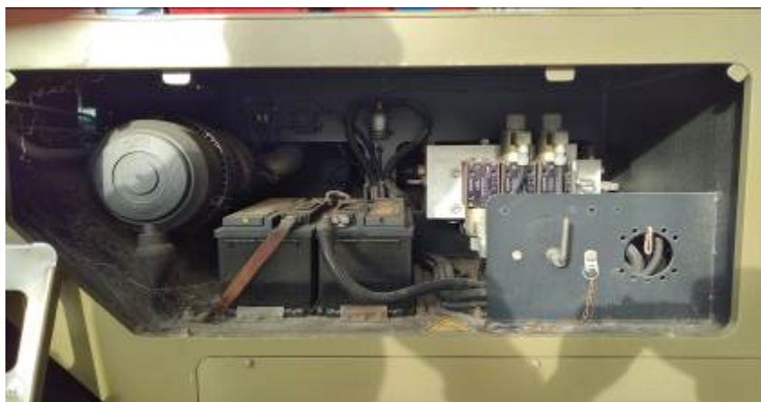
Figure 48C-6: SCHOPF F110 Tow Motor - Battery Bay (Upper Left-Side Panel)
