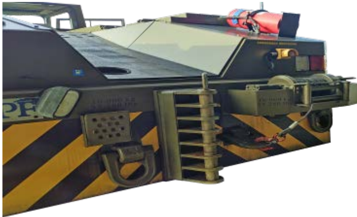
Figure 48C-9: SCHOPF F110 Tow Motor - Winch Assembly
