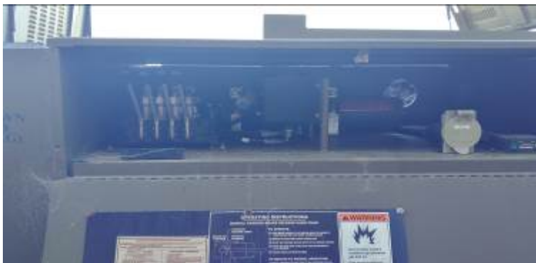
Figure 48D-9: TUG U30 Upper Right-Side Panel – Auxiliary Hydraulic Controls
