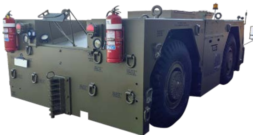
Figure 48D-4: TUG U30 Tow Motor - Fire Extinguishers
