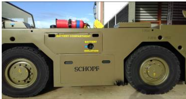
Figure 48C-3: SCHOPF F110 Tow Motor - Left Side Ballast Compartment (Lower)
