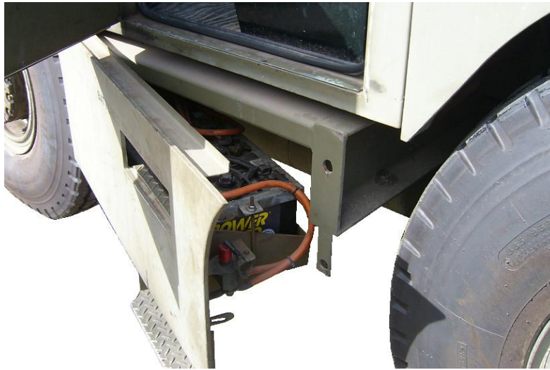
Figure 48B-3: Douglas Tow Motor's Battery Bay
