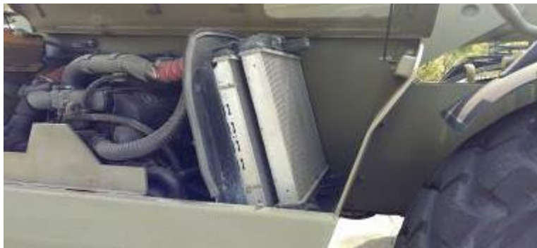
Figure 46-14: Engine Bay Condenser/Compressor
