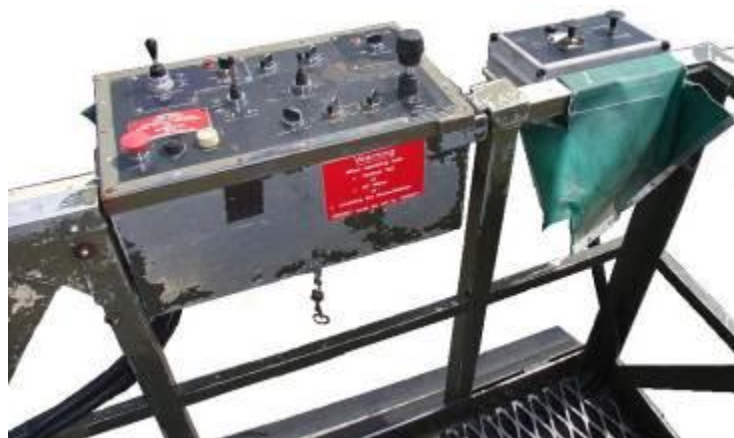
Figure 46-3: Telescopic Boom Lift's Hydraulic Control Panel
