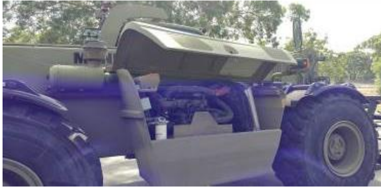
Figure 46-13: Tractor Boom Lift Manitou – Engine Bay Right Side
