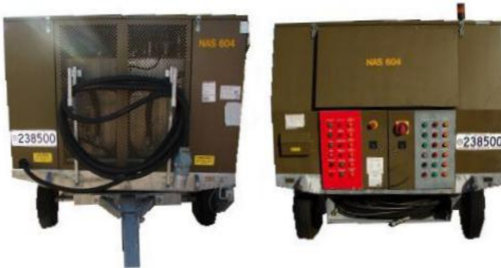
Figure 49D-3: Berendsen 10 GPM Hydraulic Rig Front (Left) and Rear (Right) Views
