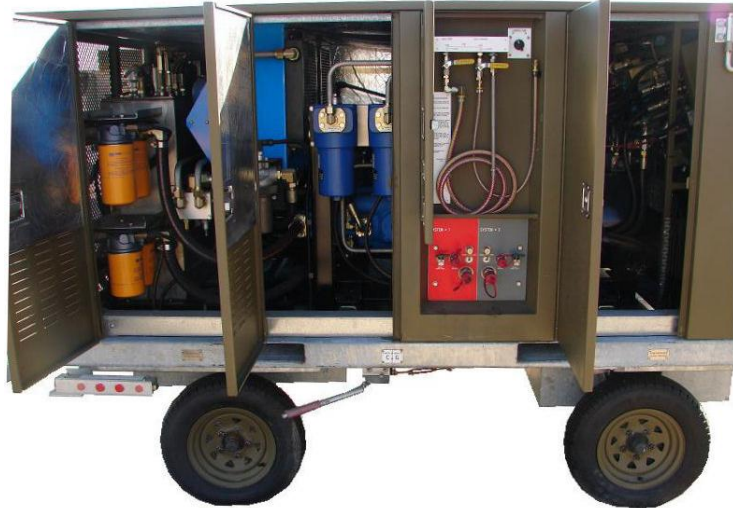
Figure 49D-7: Berendsen 10 GPM Hydraulic Rig Right Side Doors Open
