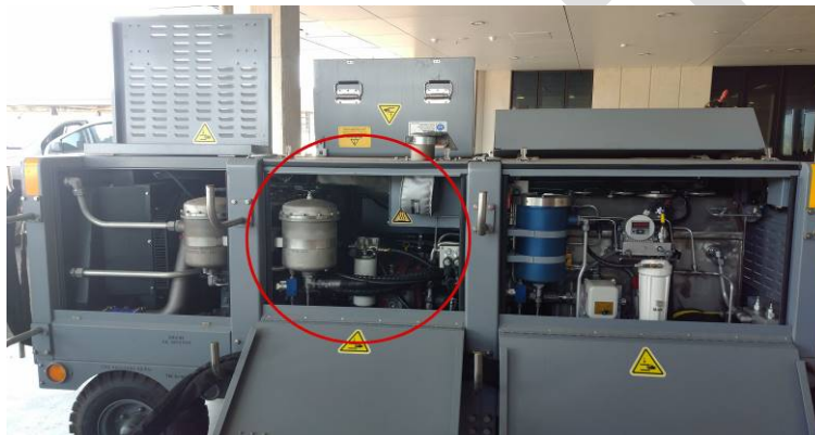
Figure 49E-7: JSF Aircraft Hydraulic Unit – Hydraulic Pump Centre Panel (Circled)
