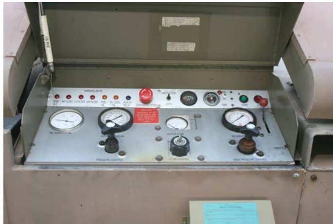
Figure 49A-5: ADP 5028 Aircraft Hydraulic Unit's Control Panel
