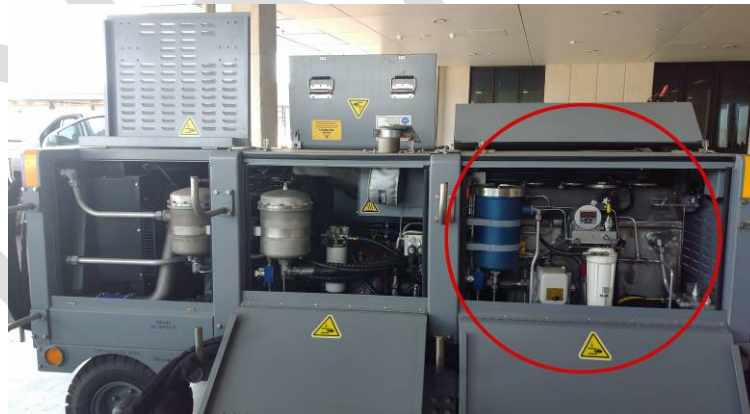
Figure 49E-8: JSF Aircraft Hydraulic Unit – Hydraulic Reservoir – Rear Panel (Circled)
