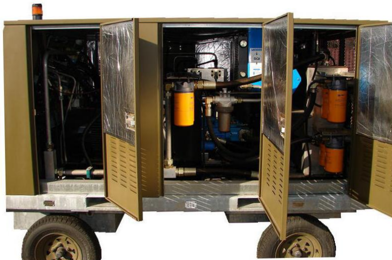
Figure 49D-9: Berendsen 10 GPM Hydraulic Rig Left Side Doors Open
