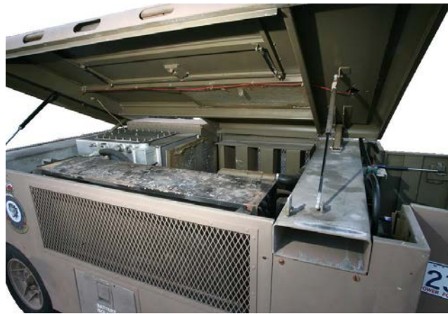
Figure 49A-7: ADP 5028 Hydraulic Unit's Engine Bay
