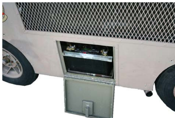
Figure 49A-2: ADP 5028 Hydraulic Unit's Battery Box
