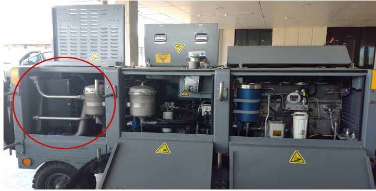
Figure 49E-6: JSF Hydraulic Unit – Front Engine Bay Panel (Circled)
