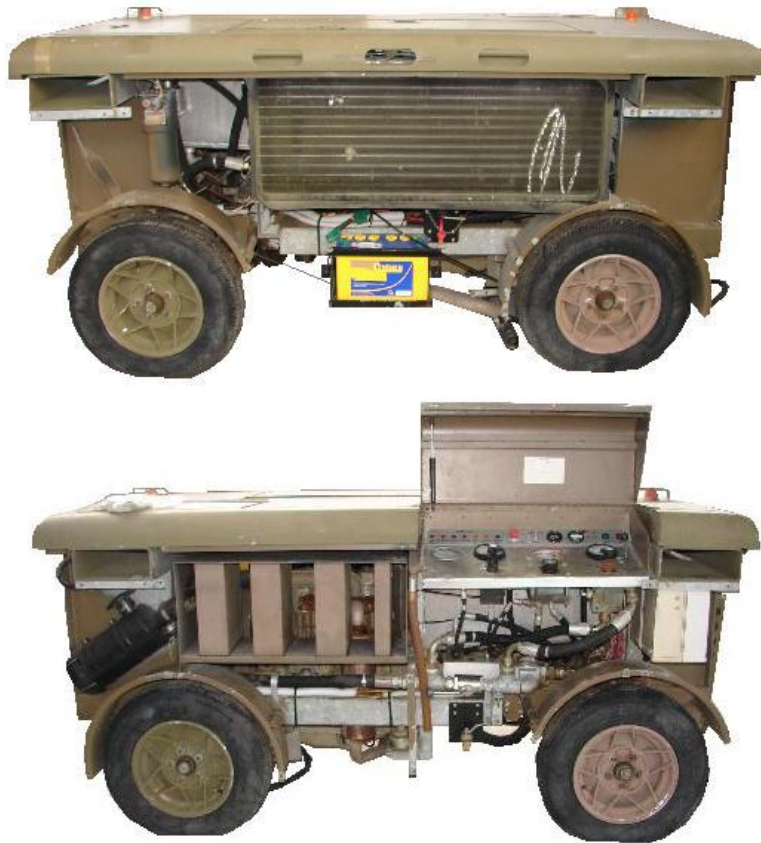
Figure 49A-3: ADP 5028 Hydraulic Unit with Canopy removed
