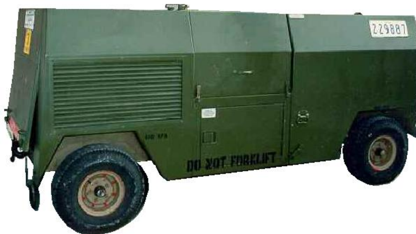
Figure 49C-1: Rexroth 35GPM Hydraulic Rig Unit
