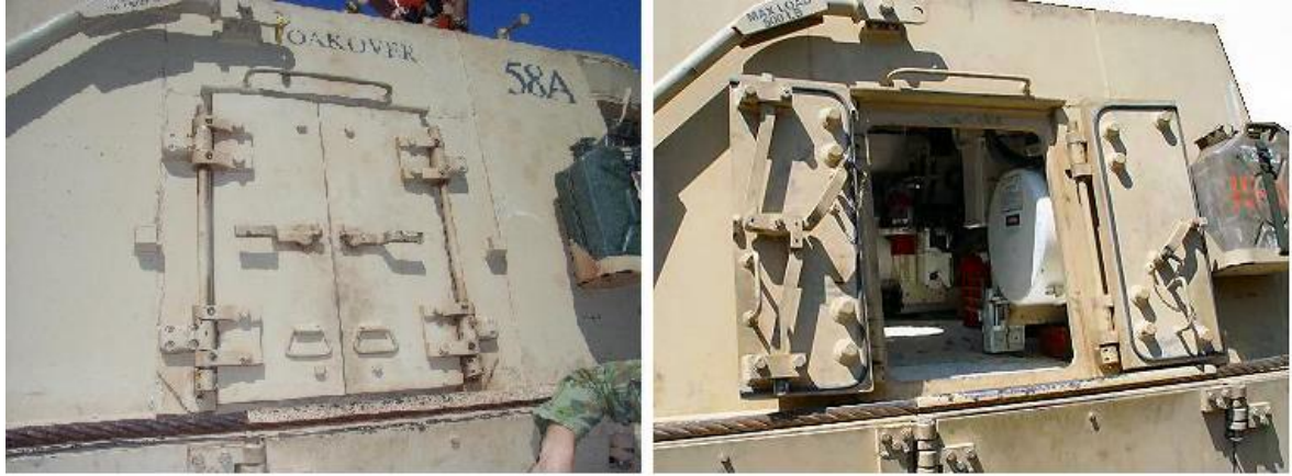
Figure 90-46: M88A2 Hercules HRV Main Entrance/Side Doors
