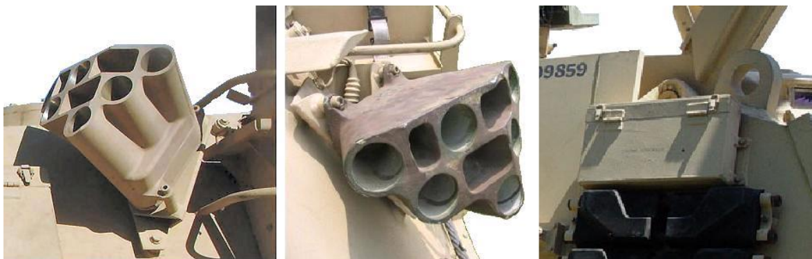
Figure 90–12: M88A2 Hercules HRV Six-barrel Smoke Grenade Launcher (Smoke Grenade Storage Box Far Right)
