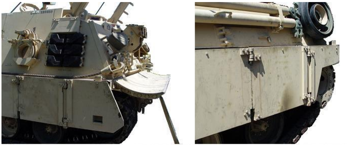
Figure 90-6: M88A2 Hercules HRV Side & Front Track Ballistic Armoured Skirt (Left) and Side Track Ballistic Armoured Skirt (Right)
