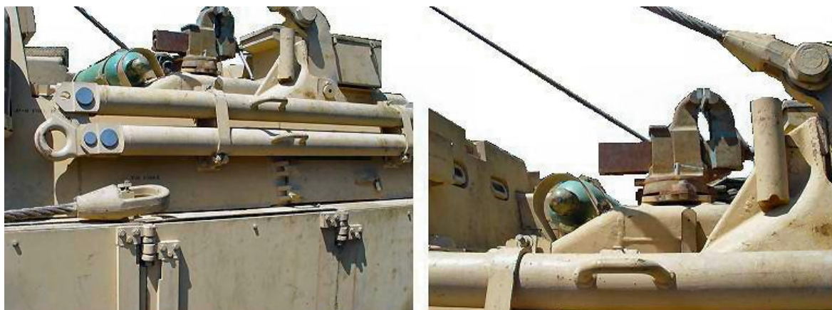
Figure 90–8: M88A2 Hercules HRV A-Frame/Tow bar and Cable Attachments (Left) Mounted Vice (Right)
