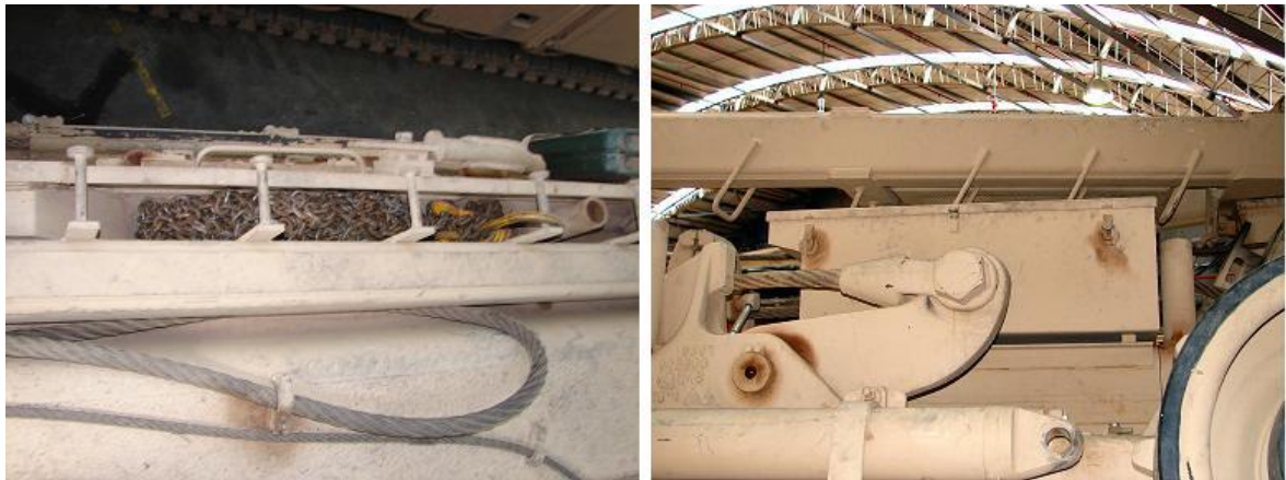
Figure 90–11: M88A2 Hercules HRV Drivers Compartment Roof Stowage Bin (Left) and Boom Tool Box (Right)
