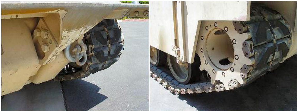
Figure 90–21: M88A2 Hercules HRV Forward Track (Left) and Rear Sprocket Hub Assembly (Right)
