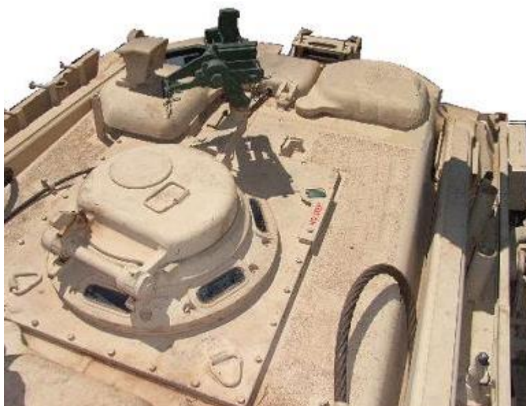
Figure 90–9: M88A2 Hercules HRV Main Cupola
