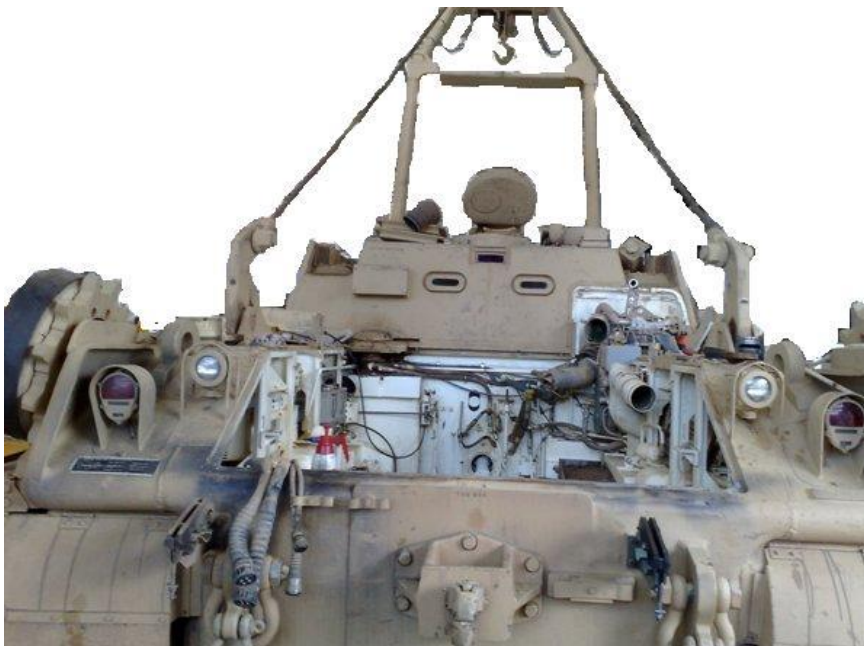
Figure 90–34: M88A2 Hercules HRV Engine Bay with armoured cover removed
