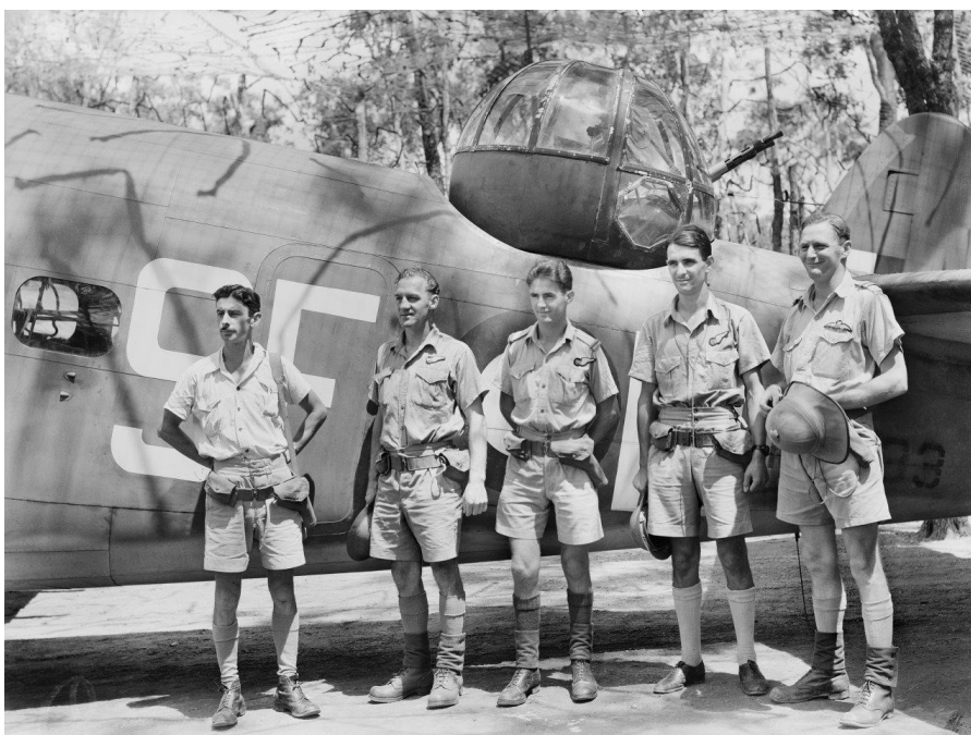
This is 13SQN's A16-233/SF-N. Note the absence of the ASV Search Array on the fuselage side. [AWM image NWA0074].
