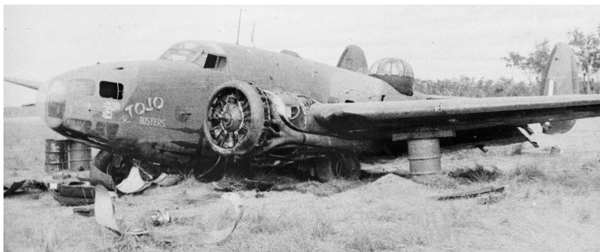
Mounted on drums, weapons removed and the detritus collected. [AWM image P00296.059]
