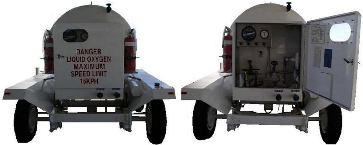
Figure 55-5: Oxygen Trailer 500 Gallon Control Cabin
