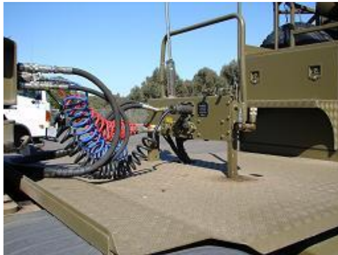
Figure 91-14: Prime Mover Hydraulic and Air Lines
