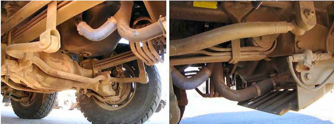
Figure 91-15: Prime Mover's Front Wheels Suspension and rear of Bumper/Scrape Guard
