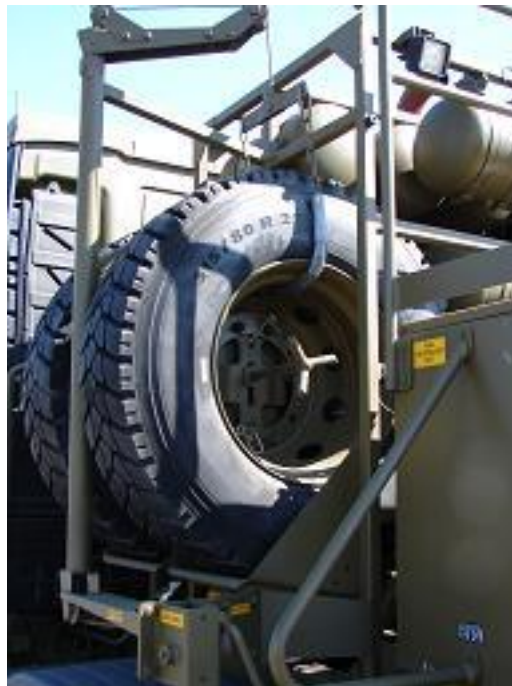
Figure 91–11: Prime Mover Spare Tyre Mount and Winch
