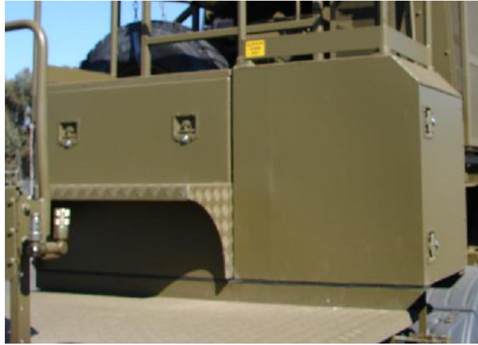
Figure 91-4: Prime Mover Main Storage Bins
