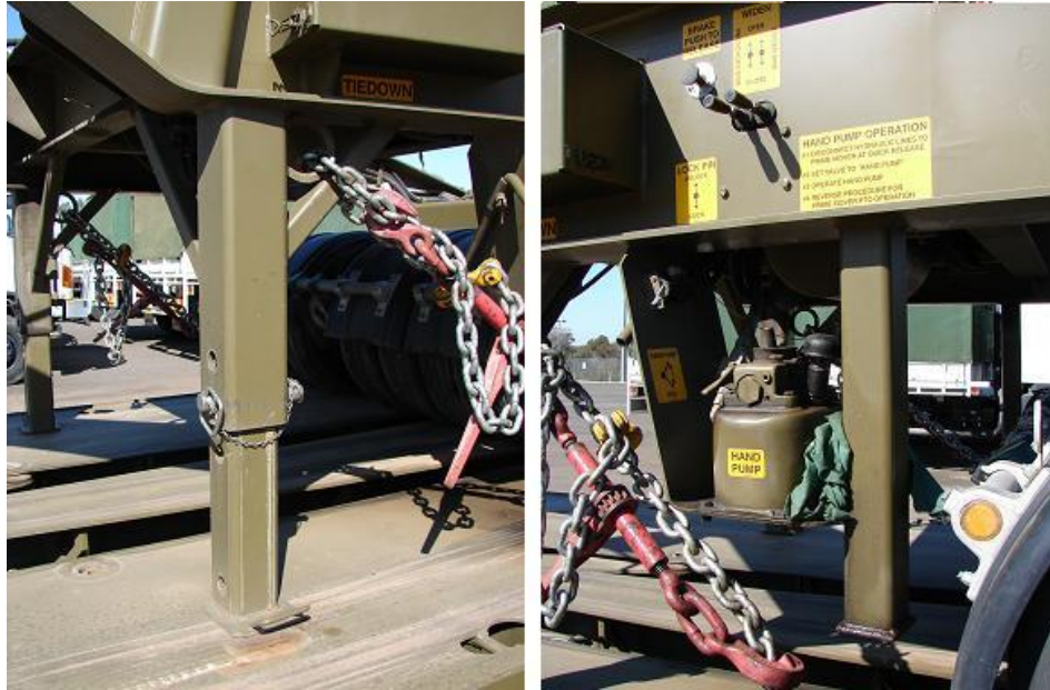
Figure 91-22: Expanding Dolly Converter Support Stand Left Side (Left) and Right Side (Right)
