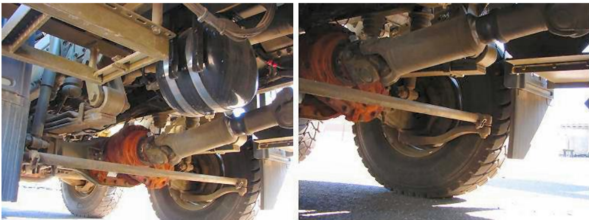
Figure 91-16: Prime Mover's Front Wheels Suspension and Tail-shaft
