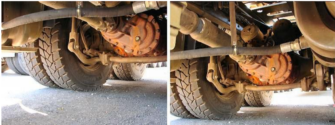
Figure 91-17: Prime Mover's Rear Wheels Suspension and Differential
