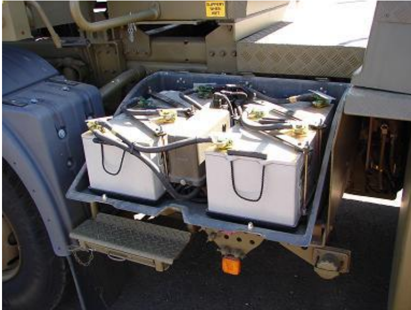
Figure 91–10: Prime Mover Battery Bay
