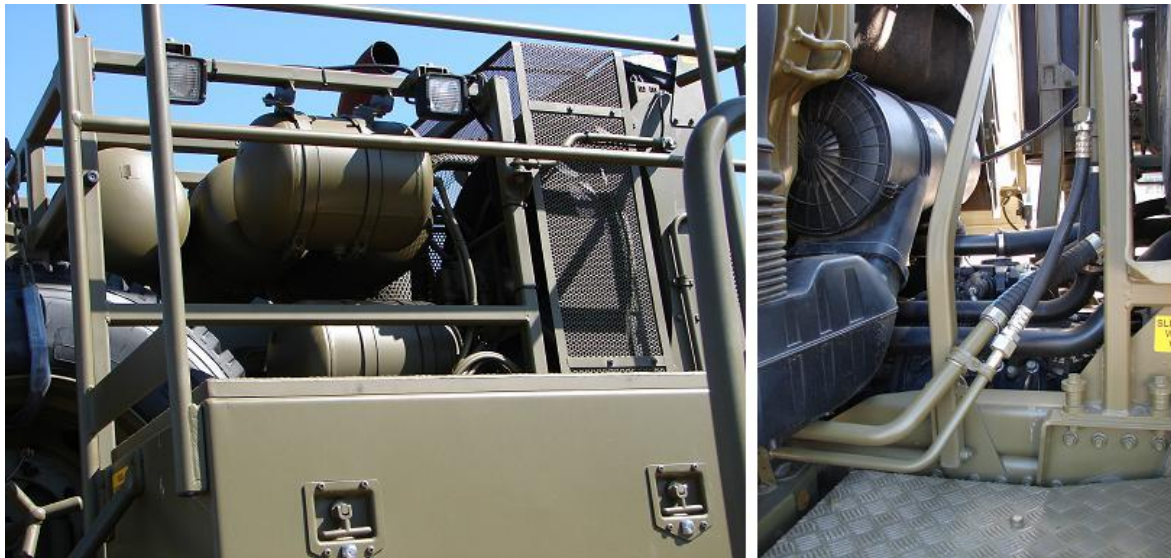
Figure 91-13: Prime Mover Hydraulic and Air Lines
