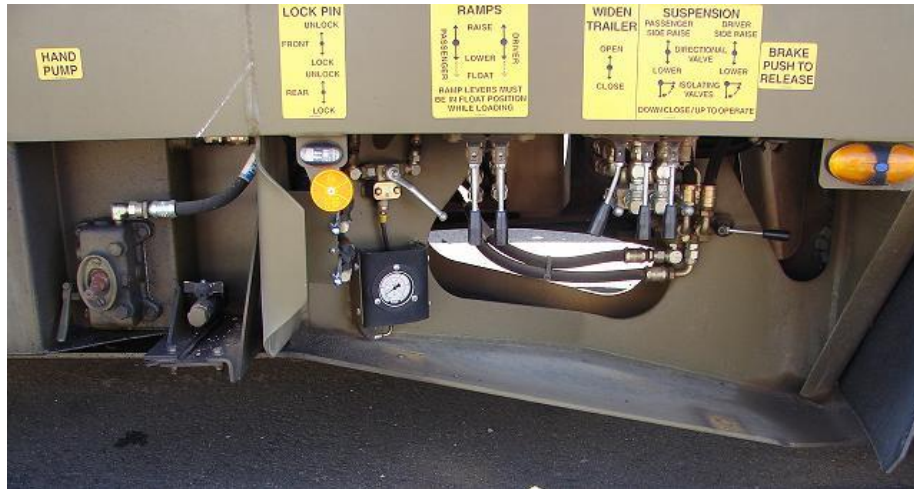
Figure 91-34: Drake Swing-wing Trailer's Hydraulic Controls
