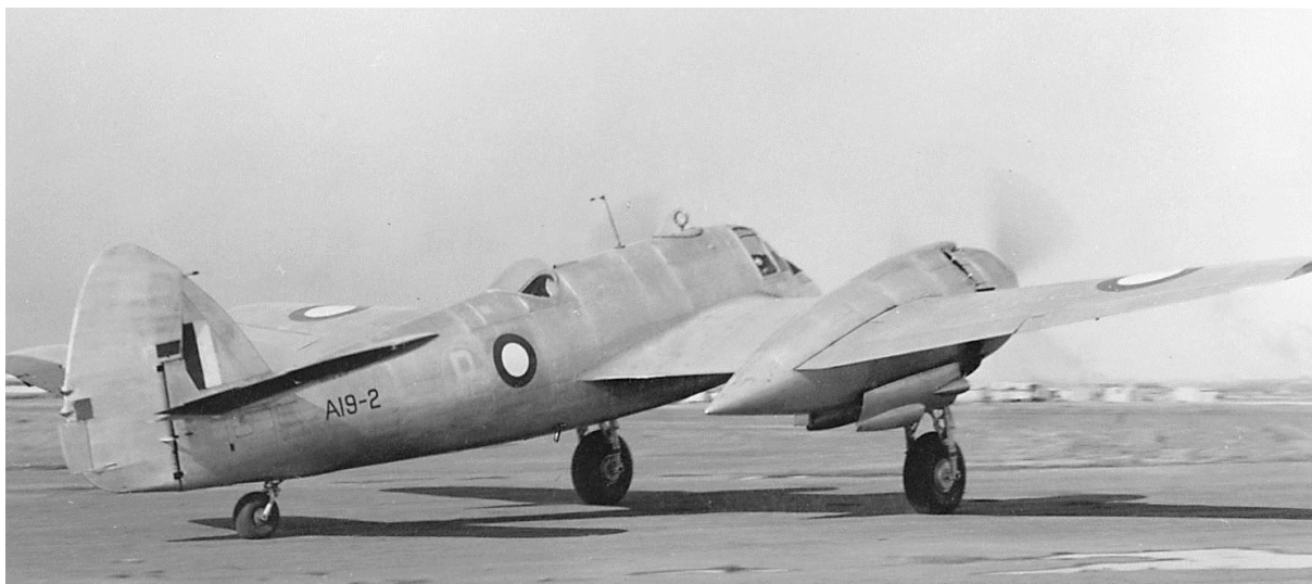
A19-2 seen here at Fishermans Bend, Victoria, with the 12° dihedral horizontal stabilisers and Wright R-2600 Twin Cyclone engines. [ADF-Serials Gallery].
