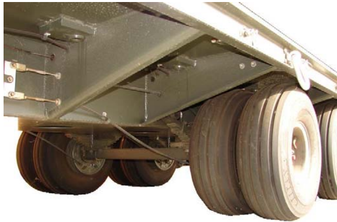
Figure 58–4: Aircraft MHU-110 Munitions Trailer's Suspension
