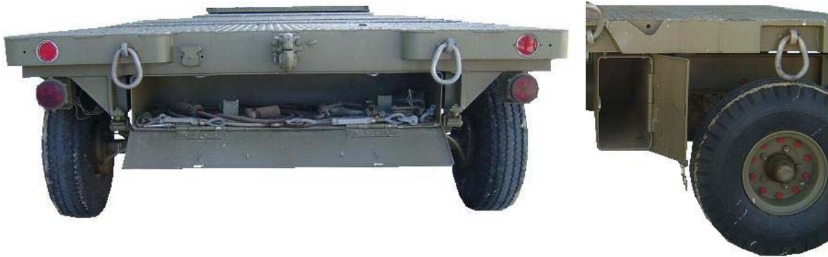
Figure 58-6: Aircraft MHU-141 Munitions Trailer Rear and Side Compartments
