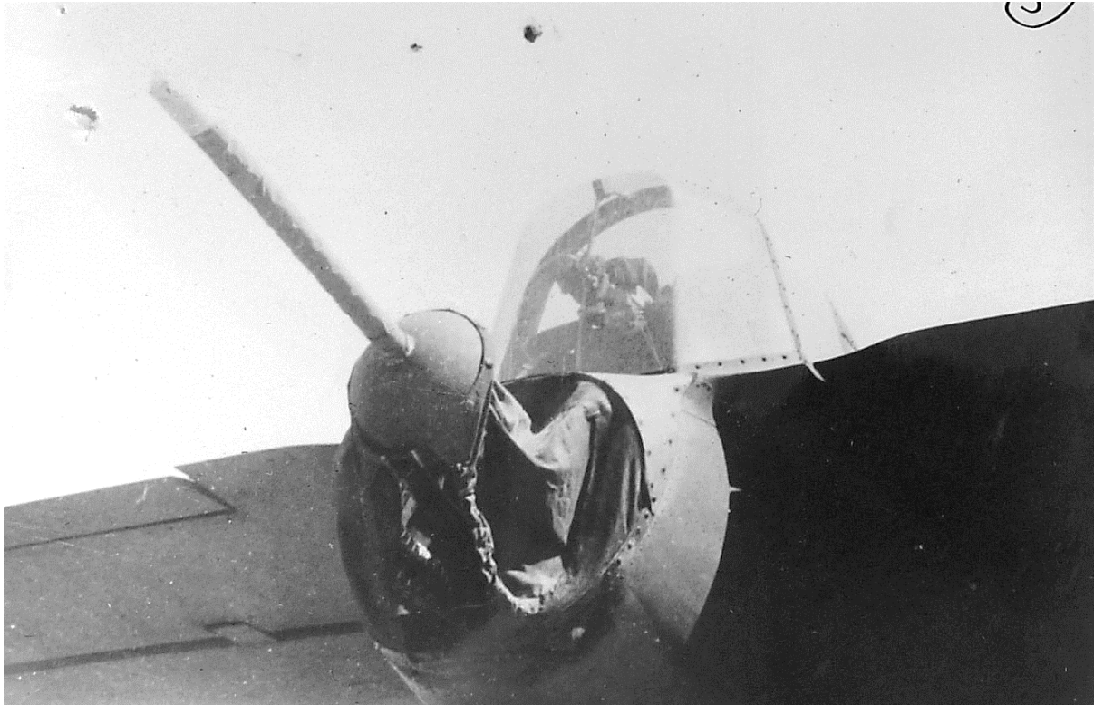
The tail gunner's position. Again, factory made, the modification centre installed the gun and some interior fittings. [NAA: A11093, 452/A47].
