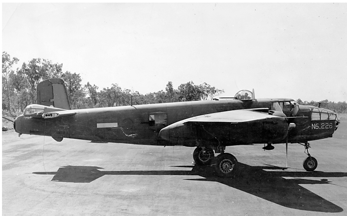
N5-226 on the ground at Darwin after losing its starboard vertical stabilizer. [Aviation Heritage Museum of WA image P901608 via Mike Mirkovic].
