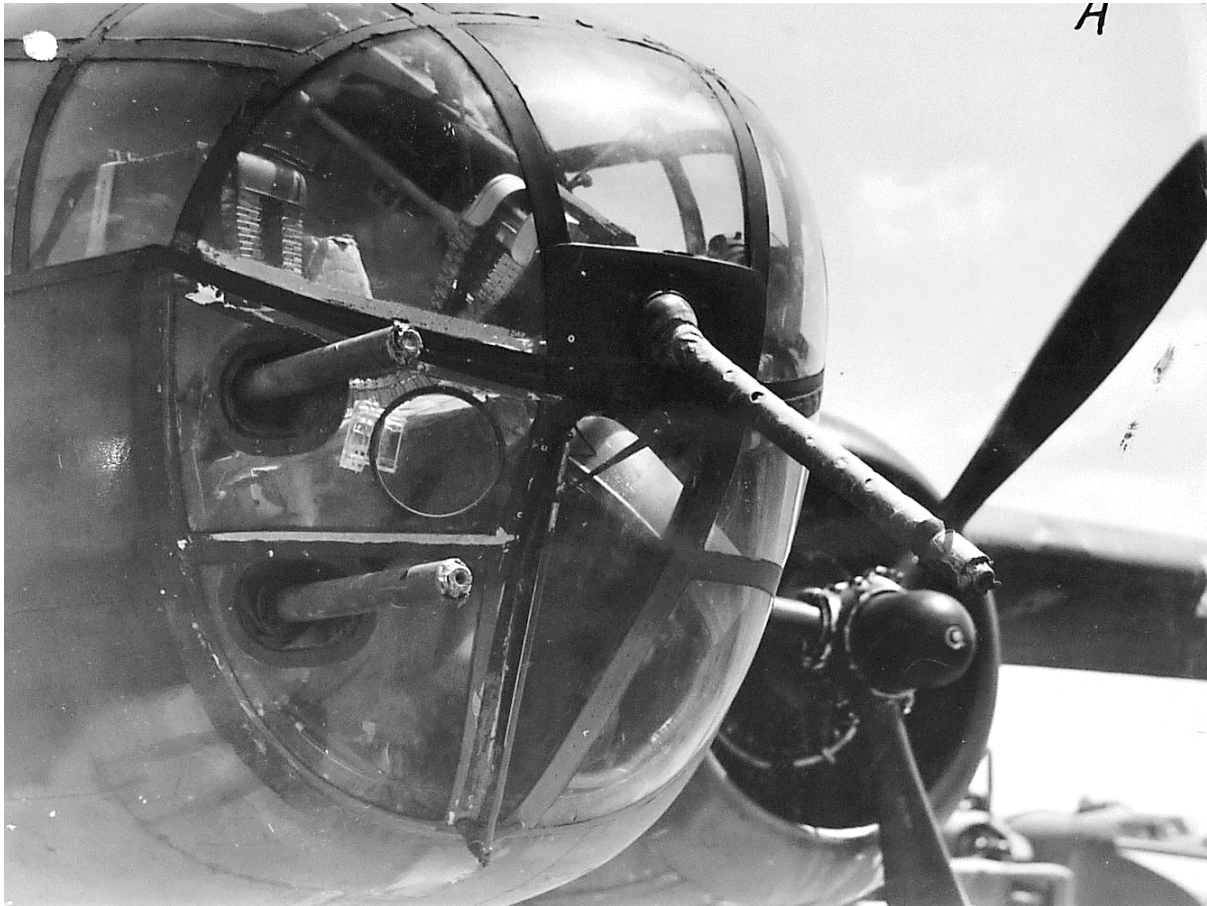
One of a sequence of close-up detail shots illustrating the external differences between B-25D-25-NC (i.e. North American Aviation model NA-100) aircraft and previous models. This one is showing the second fixed forward firing machine gun making two fixed and one flexible nose mounted guns. [Image in B-25 Aircraft North American Mitchell A47; NAA: A11093, 452/A47].
