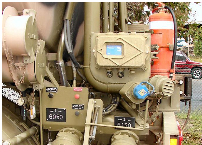
Figure 95B-10: Actros Fuel Tanker's Pump Control Panel
