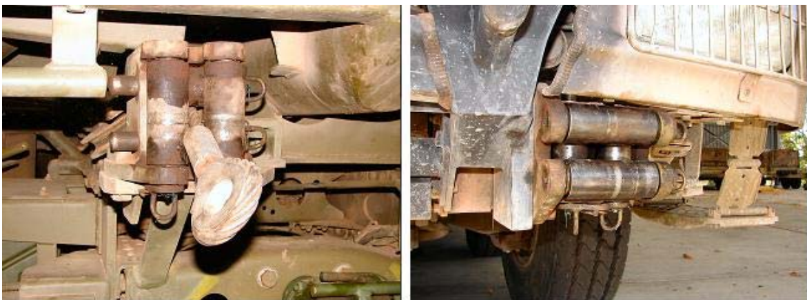
Figure 95A-7: Actros's Gantry's Winch Rollers Rear (Left) and Front (Right)
