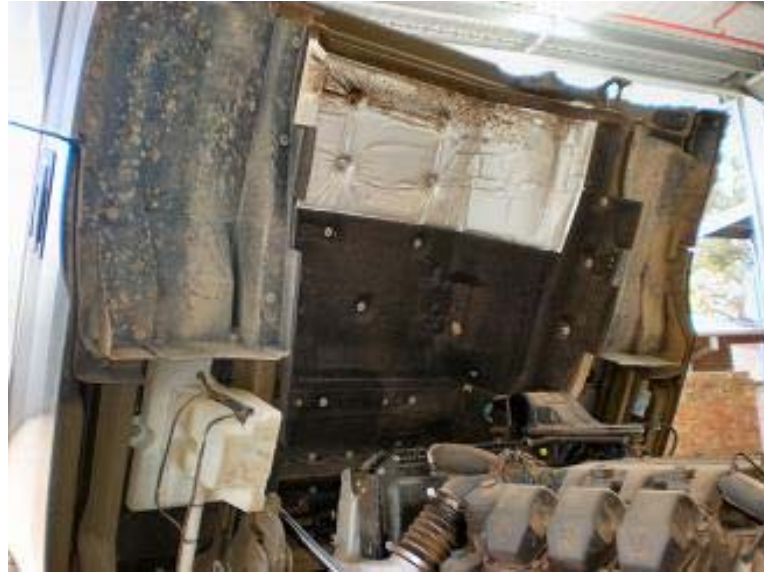
Figure 95-25: Actros Engine Bay Heat Suppressant
