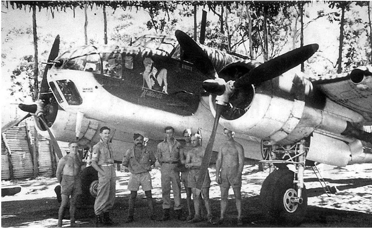
Forward quarter view of 2SQN's A9-576/KO-Z. The name, nose art and bomb log are visible from this aspect; also the typical style ASV Homing array – no Yagi aerials under the wings. [Image via Kas Grigonis, ADF-Series facebook page].
