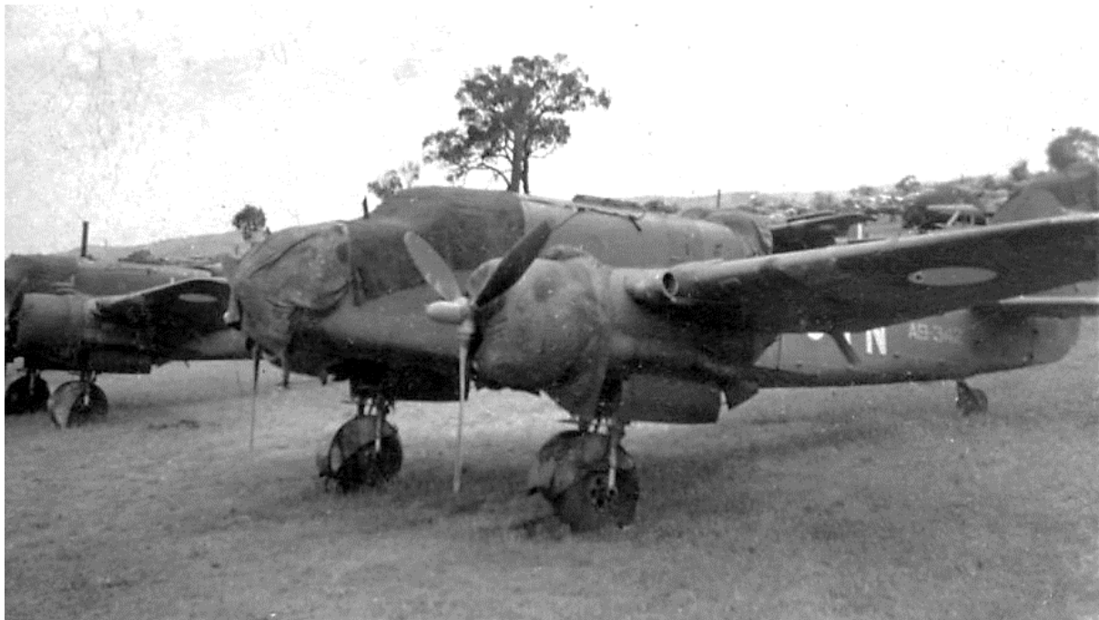
A9-342, in storage post-war at 5AD FOREST HILL. It is wearing the later war standard over-all RAAF Foliage Green (K3/177). Serial number is RAAF Medium Sea Grey (K3/183) and the code letters, seem to have been Sky Blue. [Mike Mirkovic via adf-serials].
