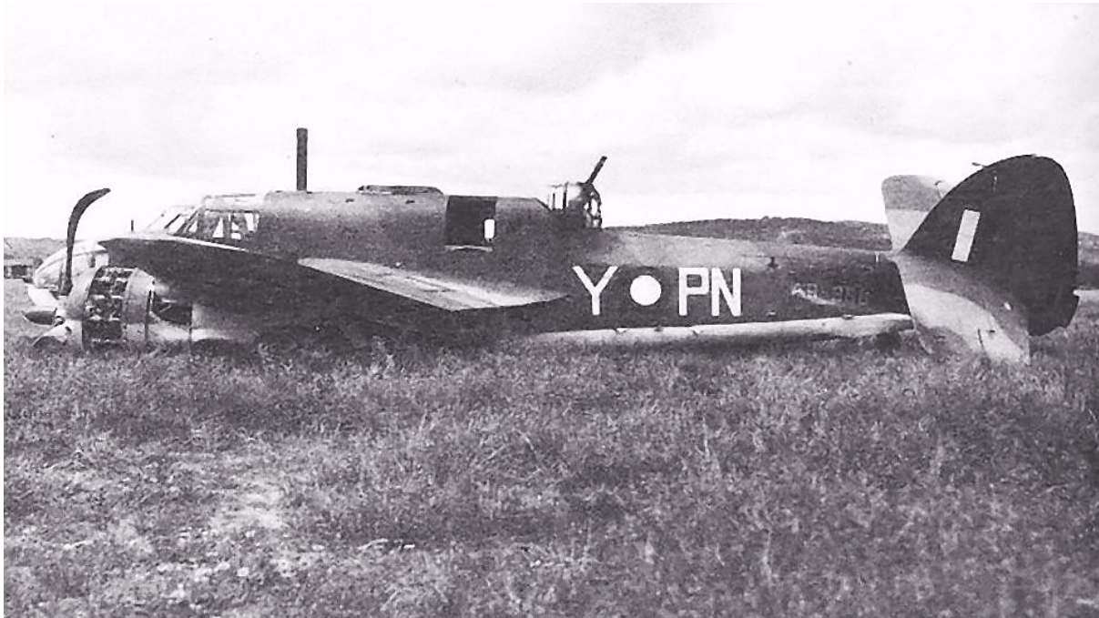
The adf-serials caption for this image says it is “A9-385”. It is, in fact, A9-358. The “twisting of the rear fuselage” mentioned in the text, above, is obvious in this image. [Mike Mirkovic via adf-serials].
