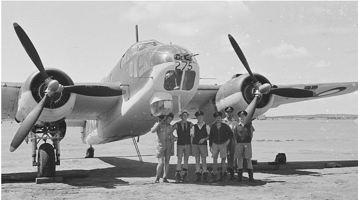
A9-275, PN-X. ASV Homing TX whiskers prominent. [National Archives of Australia NAA: A14435, LA/115].
